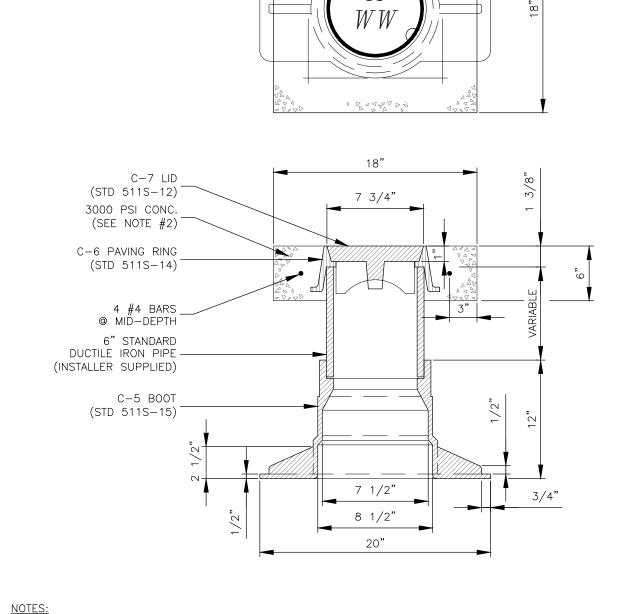
NUMBERED CASTINGS STANDARDS SHOWN IN PARENTHESES ARE REFERENCES TO THE CITY OF AUSTIN STANDARDS CRITERIA MANUAL. DELETE CONCRETE & REBAR WHEN VALVE IS WITHIN PAVED STREET.
