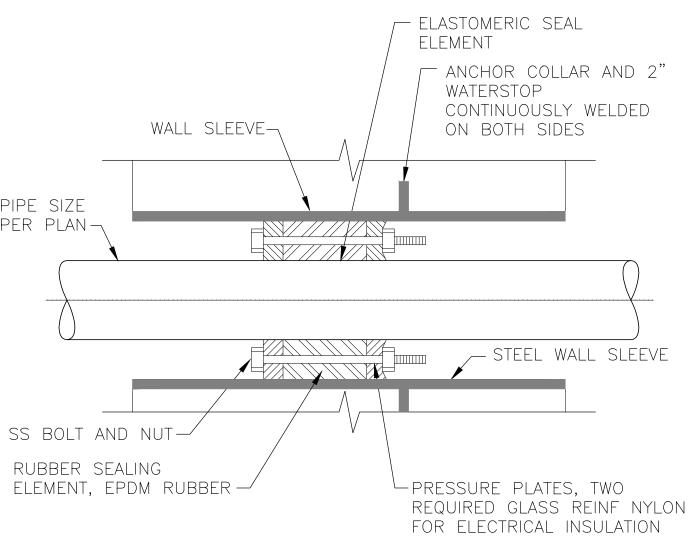
. INSIDE DIAMETER OF EACH WALL OPENING SHALL BE OF THE SIZE RECOMMENDED BY THE MANUFACTURER TO FIT THE PIPE AND THE WALL SEAL ASSEMBLY TO ASSURE WATER-TIGHT JOINT.
