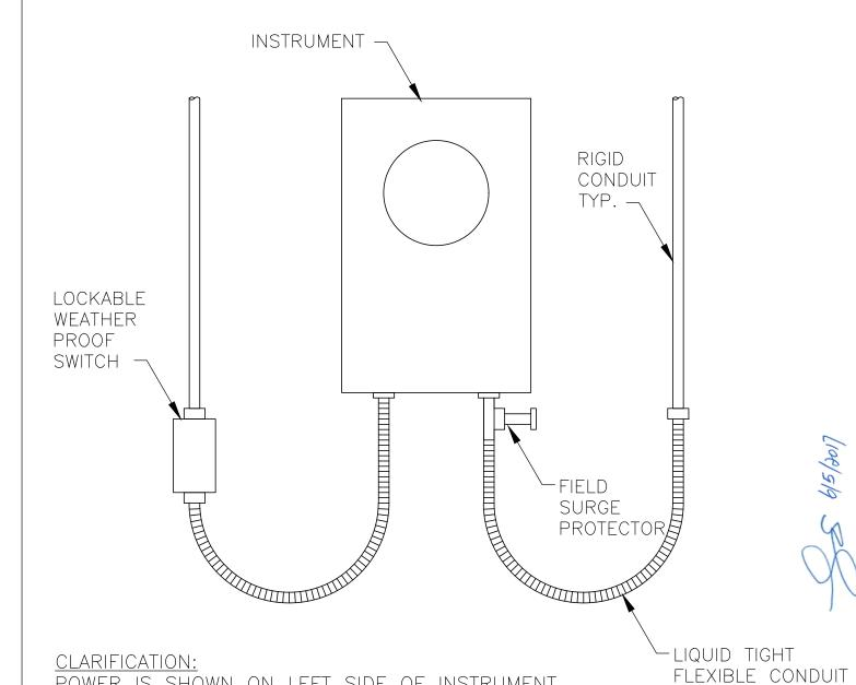
POWER IS SHOWN ON LEFT SIDE OF INSTRUMENT WITH A DISCONNECT AND ANALOG ON RIGHT SIDE WITH SURGE PROTECTOR. FIELD SURGE PROTECTOR — PHOENIX CONTACT SURGETRAP EX OR APPROVED EQUAL.
