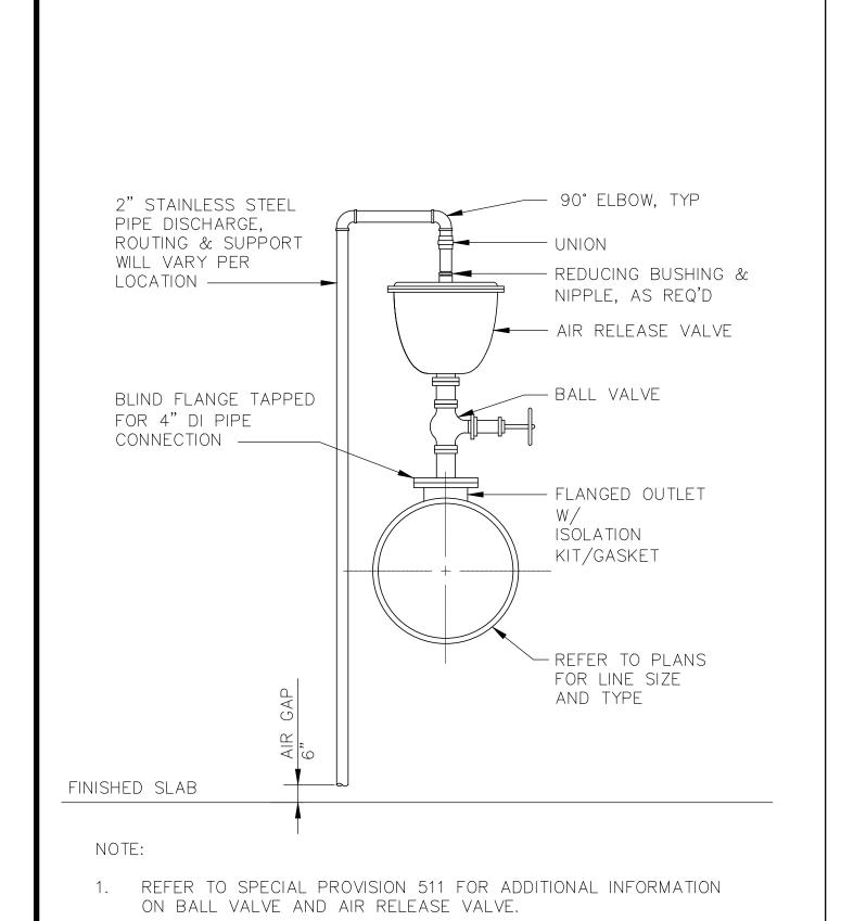
COMBINATION AIR VALVE -UNION — — TAP FLANGE FOR THD CONNECTION BALL VALVE-4" FLANGED OUTLET, SERVICE SADDLE OR TAPPED PIPE REFER TO PLANS 2" STAINLESS STEEL FOR LINE SIZE PIPE DISCHARGE, AND TYPE-ROUTING & SUPPORT WILL VARY PER LOCATION FINISHED SLAB NOTE:
