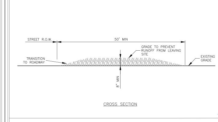
3. LENGTH SHALL BE A MINIMUM OF 50' FROM ACTUAL ROADWAY, AND WIDTH NOT LESS THAN FULL WIDTH OF
