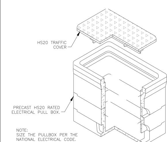
HAND HOLE FOR FIBER OPTIC CABLES
