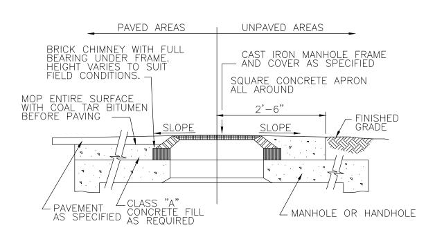
FINAL GRADING SHALL PROVIDE ADEQUATE DRAINAGE AWAY FROM MANHOLE COVER IN ALL DIRECTIONS.
