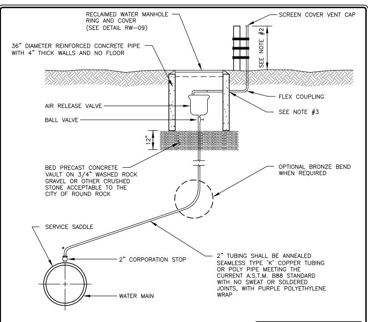
\* THREAD TO COMPRESSION BRASS ELBOW ALLOWED IF NECESSARY DUE TO DEPTH LIMITATIONS
