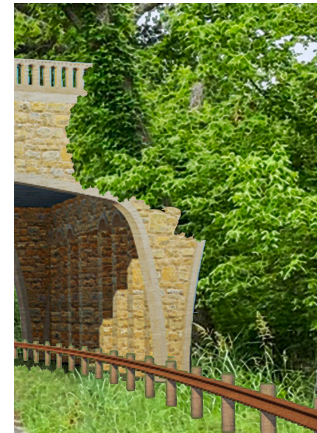
Option 3 Sloping facade with stone pattern *requires guard fence on north side of road
