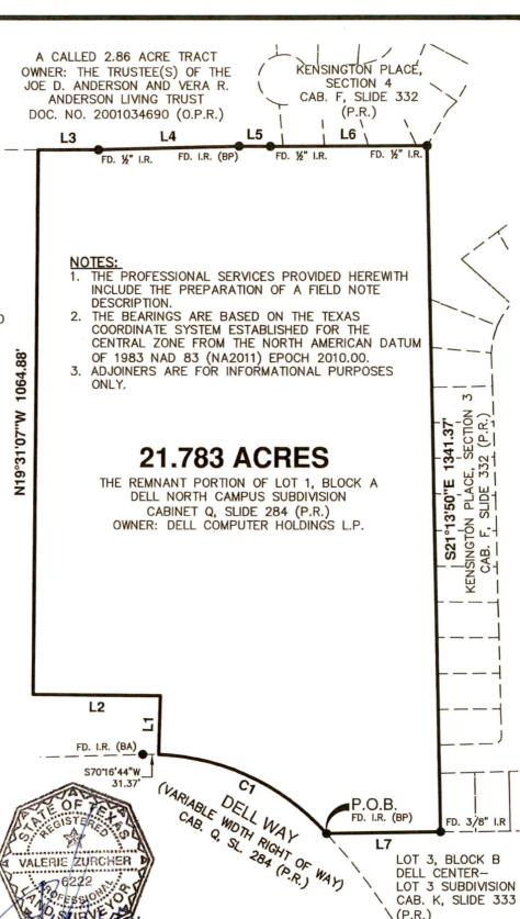
LINE TABLE LINE **BEARING** LENGTH L1 N18'26'37"W 114.89 S70'30'50"W 12 251.00 L3 N70'00'24"E 118.51 N68'30'24"E L4 277.22 L<sub>5</sub> N70'25'52"E 61.98 N69'50'23"E 16 306.17 S69'04'34"W 222.44
