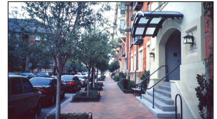
Sidewalk appropriate for Round Rock's retail areas with tree planters in furnishing zone, parallel to parking lane. Landscaping occupies the shy distance between the building and the sidewalk. The ground floor is elevated as privacy is important for residential units along busy streets.
