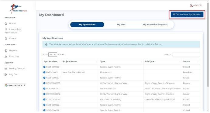
3. Application Tab: Clicking New Application to create a brand-new application. You can also add a project name at this stage. Clicking on Building Inspection Services will reveal an expandable list of all the available application types. Find the type of application you wish to submit by expanding the department's name. Select Next at the bottom of the screen to continue.
