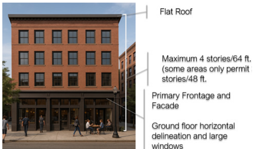
Figure 11: MU-2 Type 2 Design Features
