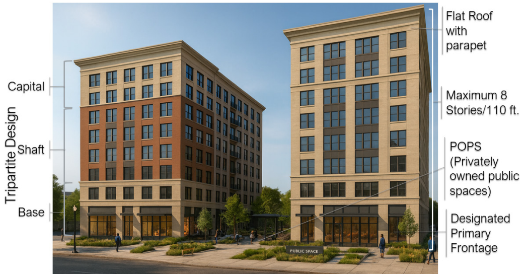
Figure 12: MU-2 Type 3 Design Features
