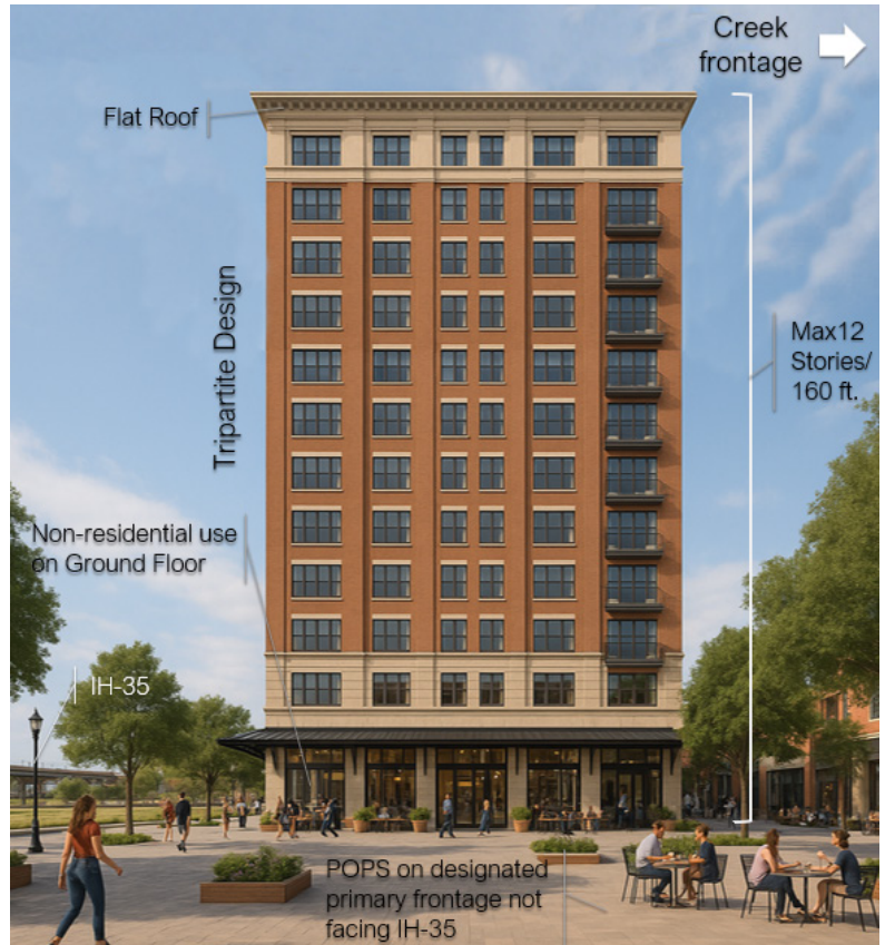
Figure 13: MU-2 Type 4 Design Features
