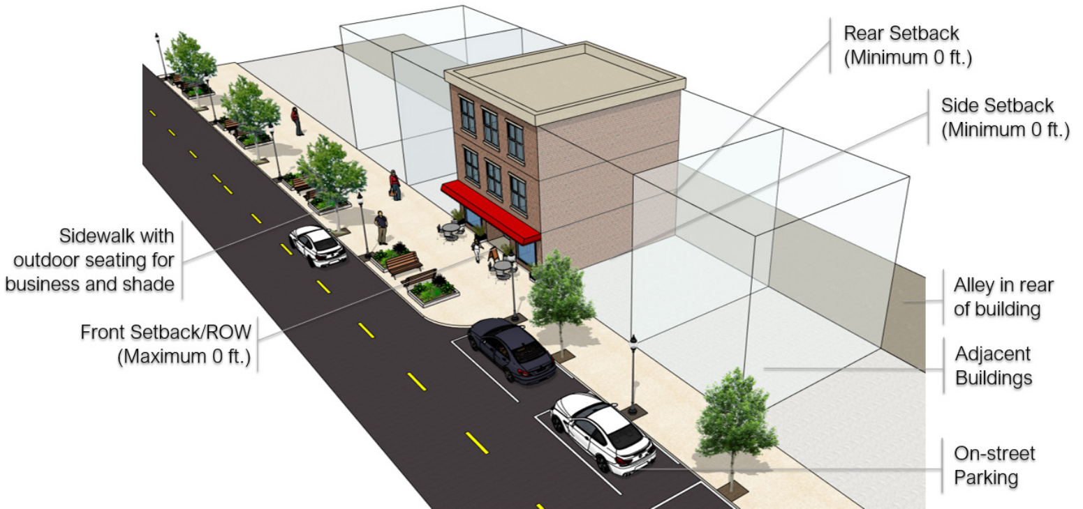
Figure 5: Setback with an alley for Principal Building
