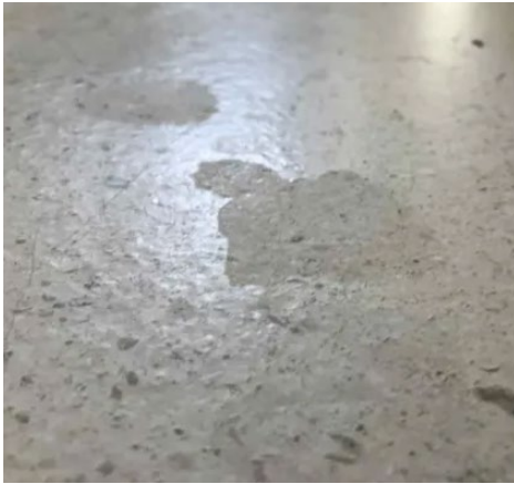
Limestone floor tile etched by citric acid
