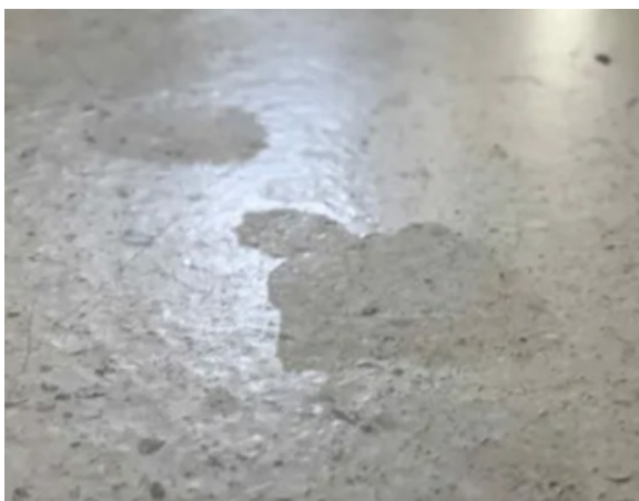
Limestone etched by citric acid
