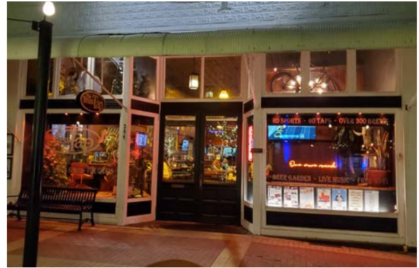
Storefronts feature large display windows. (Left) Transom windows above helped to direct light toward the back of the building, as the side walls were shared with adjacent buildings.
